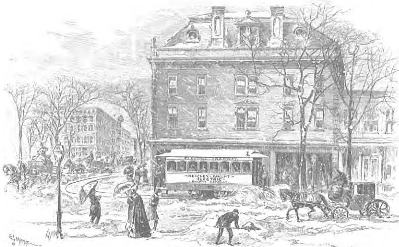
A Bentley-Knight trolley, powered by contact with an electric conduit between the tracks.
